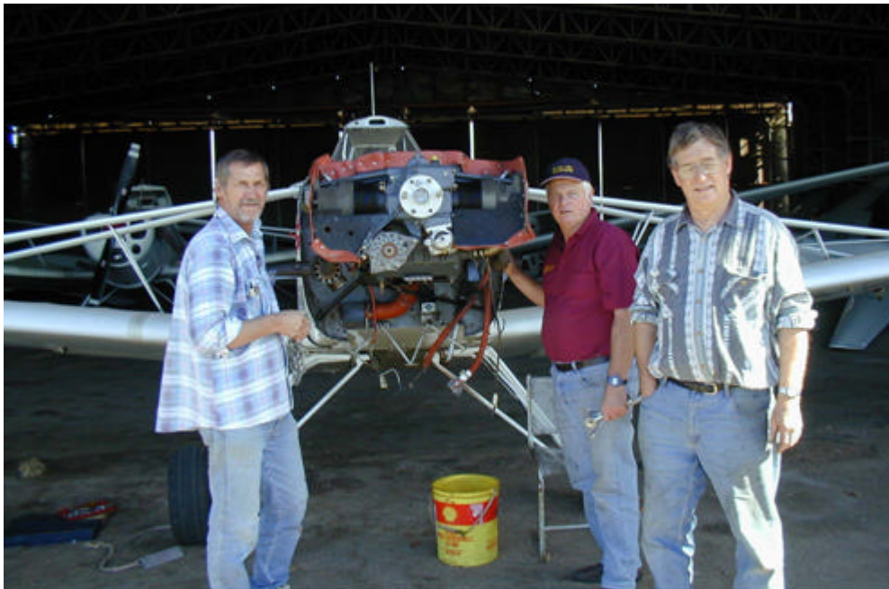
Allen Hudson, Bob Pratt and Ivor Paech having just finished securing the engine to the mountings of the Pawnee VH-WGC at the Waikerie Gliding Club
